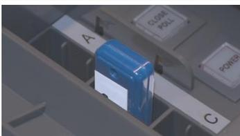
6. Remove media stick from slot **after** power button is no longer lit and place it in the clear corner pocket of the yellow return bag. Shutdown is complete.
