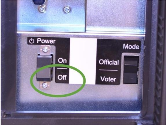
1. Unlock left side access door with barrel key and flip power switch to **Off**.
