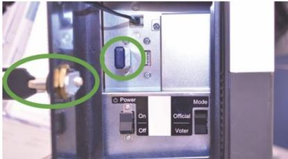
5. Use barrel key to open left side access door and verify media stick is in place.
